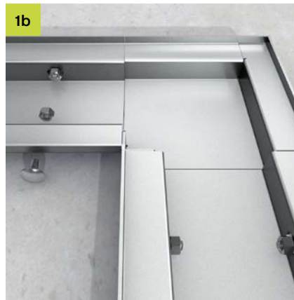
1b Then screw the L-connector and the duct segments together with FRSV 6x12 and SEMS 6 nuts.
