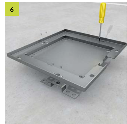
6 3 levelling anchors are required to mount the cassette. Fix with 2 countersunk screws UKS M3x6E per levelling anchor (positions see picture).
