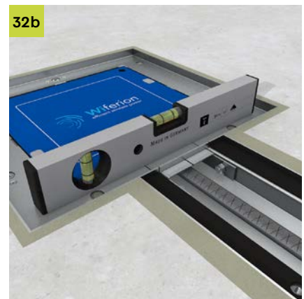
32b The quick connector must be flat with the contact surface of the cassette.
