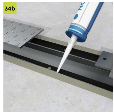
34b To protect against water and dirt, apply sealant to the edge of the heavy-duty trunking cover before inserting the heavy-duty trunking cover.
